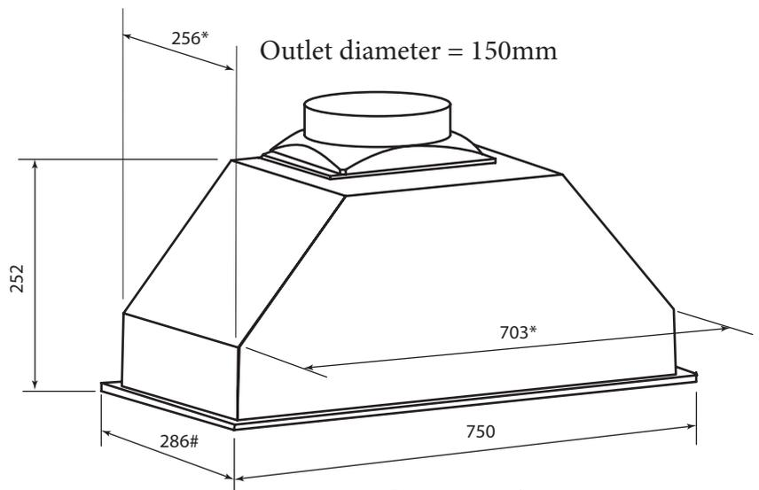
\* allow 5mm clearance for installation
