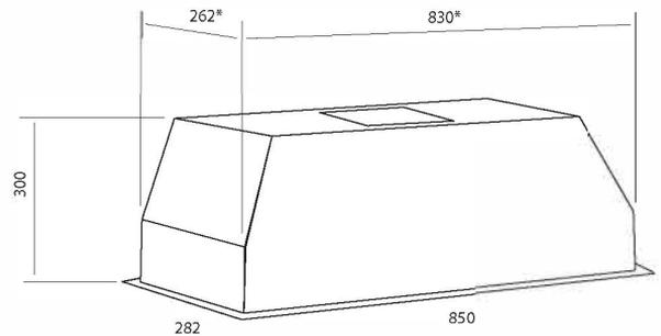
\* allow 5mm clearance for installation
